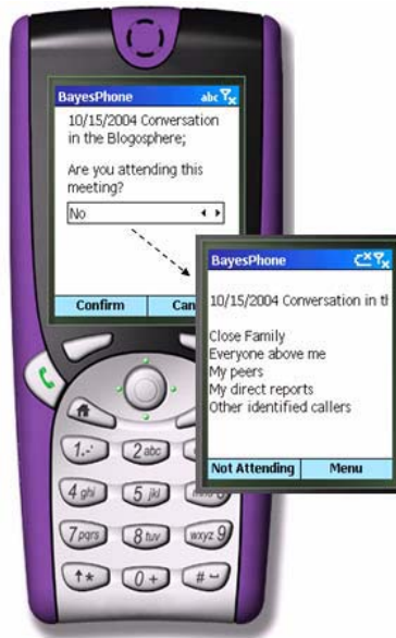
Fig. 5. Bayesphone application, showing the case where it is best to ask the user about attendance of a forthcoming meeting. When the meeting starts, the application displays the title of the meeting in progress, the input from the user, and the callers who can break through
