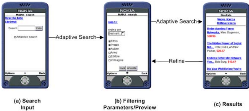
Fig. 1. The results adaptation pattern: (a) keyword search and option for requesting an adaptive result; (b) the user can preview the adaptation parameters selected by the system and eventually change them; (c) the adapted result lists displays the items with the selected features
